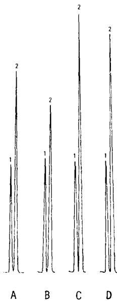
FIG. 3. Gas chromatograms of extracts from aqueous standard (A) plasma (B) urine (C) saliva (D). 1, Quinoline. 2, Nicotine.
